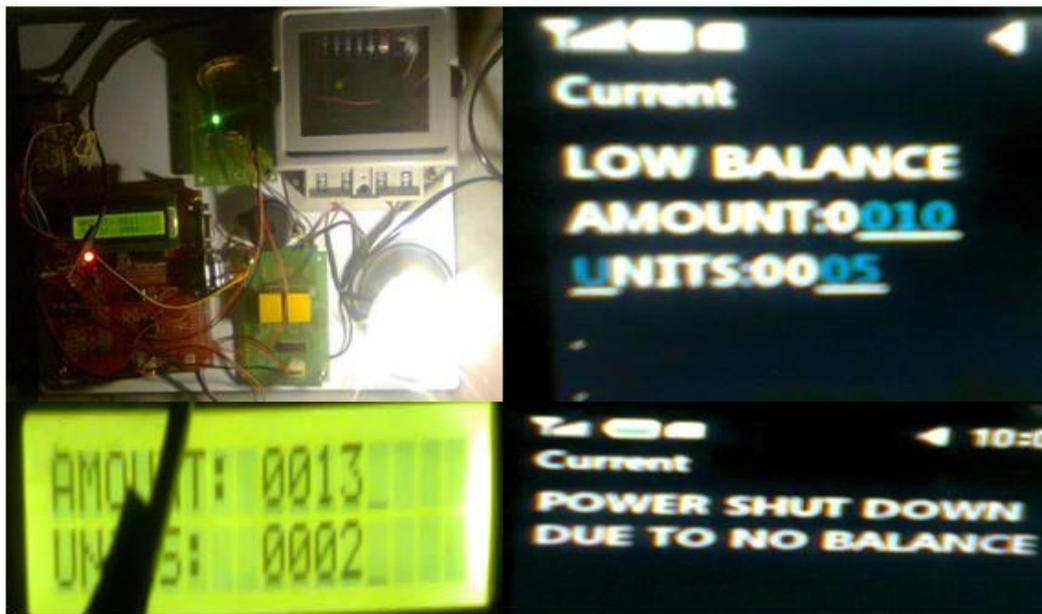
The implementation of Realization of GSM BASED AUTOMATIC ENERGY METER READING SYSTEM WITH INSTANT BILLING is done successfully. The communication is properly done without any interference between different modules in the design. Design is done to meet all the specifications and requirements It can be concluded that the design implemented in the present work provide portability, flexibility and the data transmission is also done with low power consumption.
